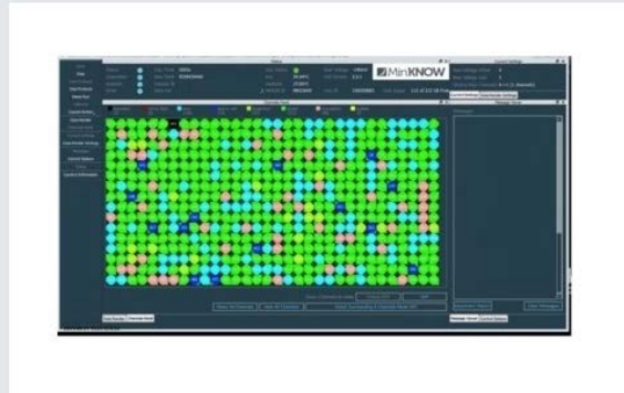
Figure LDCP: Channel Panel screen at the start of a Lambda DNA experiment. A good library will be indicated by a high proportion of light and dark green channels. The combination of light and dark green indicate the number of active pores at any point in time and the dark green indicate the proportion of pores in strand (or sequencing) at a particular time point. A low proportion of dark green channels will reduce the throughput of the sequencing.
