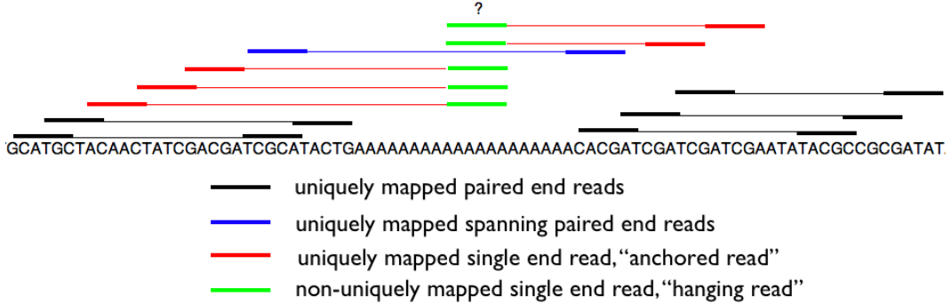
Figure 2.1: Four of the various mapping scenarios related to paired end reads. Paired end reads which map uniquely within the genome and are filtered only by their mapping quality are known as unique reads (black). Paired end reads which are of sufficient length and have mapped on either side of a repetitive region are known as spanning reads (blue). Adjacent to repetitive regions lie anchoring reads which map to the unique flanking regions of a repeat (red) and whose mate (green) maps within the repetitive region.
